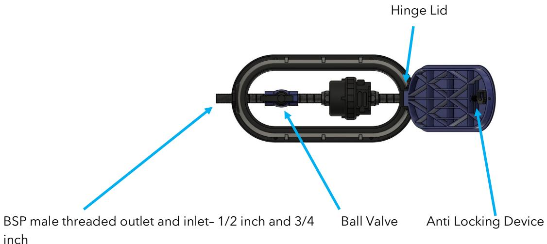
BSP male threaded outlet and inlet- 1/2 inch and 3/4 inch
